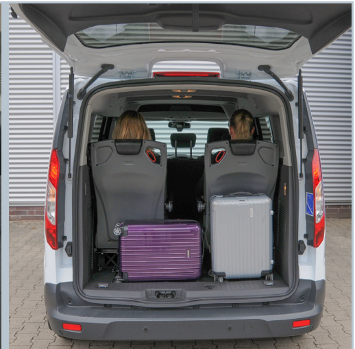
Tip & fold seats with integrated 3-point safety belt and headrest.
